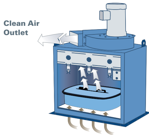
NORMAL OPERATION FOR CPV-1 MODEL
